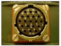
Figure 8-1 Connector Pin Out
